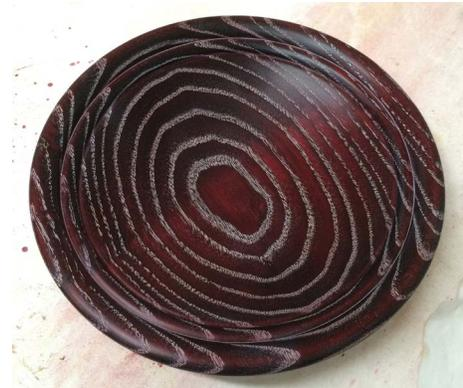
Ash bowl, 8" (20cm) diameter, before and after application of dye and liming wax.
