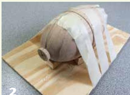
Workpiece is glued and taped to the wedges and carrier, ready to be cut apart on the bandsaw. Note the intended cut line for this pod form (along the sidegrain). The jig can also be used to cut across the grain to remove a tenon.
