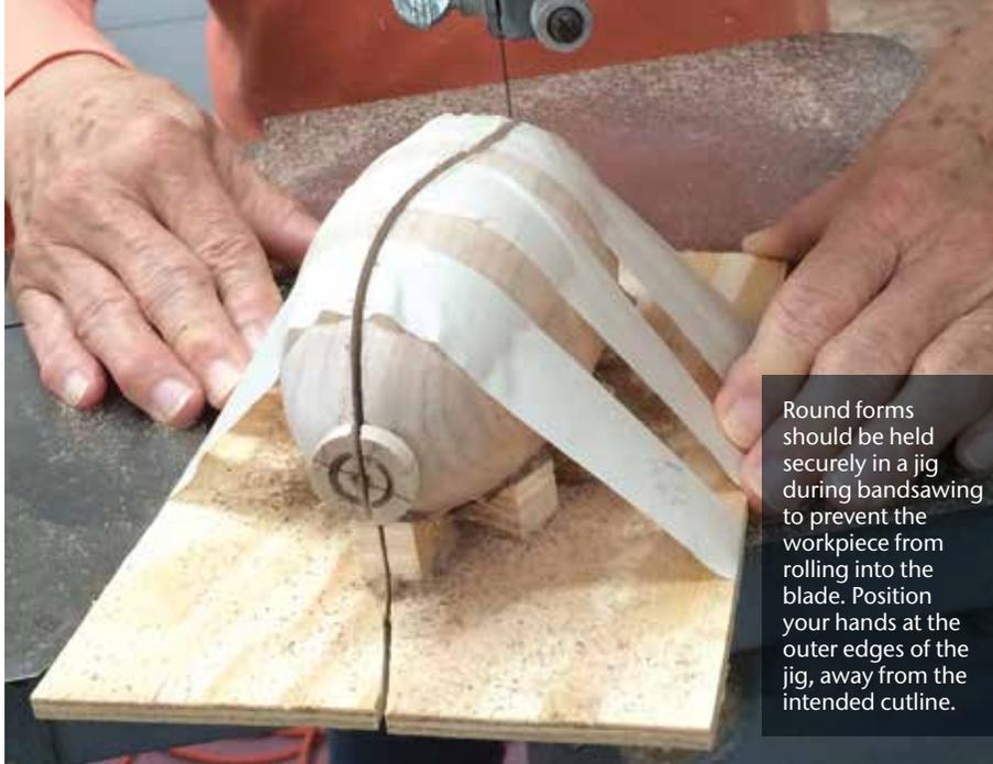
Round forms should be held securely in a jig during bandsawing to prevent the workpiece from rolling into the blade. Position your hands at the outer edges of the jig, away from the intended cutline.
