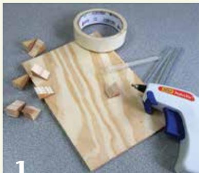
Materials needed: scrap wood, wedges, hot-melt glue gun, glue, and masking tape.
